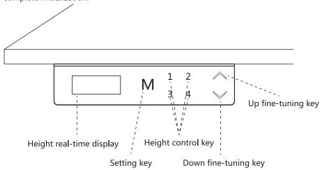
Height control key setting: Use the up fine-tuning key or the down fine-tuning key to raise or lower the height what you need. Click the setting key M and click the code to be set (any of the 1-4 height control keys) after releasing it to complete the setting. 7 . Use pan head screws to fix the handset switch to the table.
