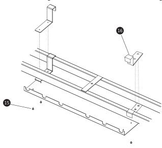
6. Place the table plate facing up horizontally, then invert the main crossbar end and buckle it upside down on the table plate.
