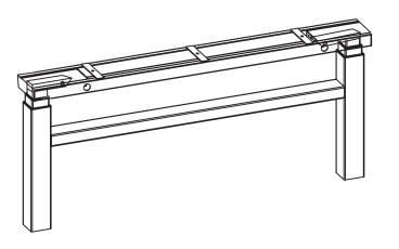
2. Align the two legs facing down to the bottom of the two stand columns, fix them with machine screws to ensure the locking is not loose, and then install the four leveling studs to the bottom of the feet.
