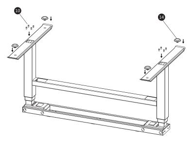
3. After installing the feet and leveling studs, put the whole frame in the right position, put two side brackets and one support bracket above the frame, and then lock it with flat head screws.
