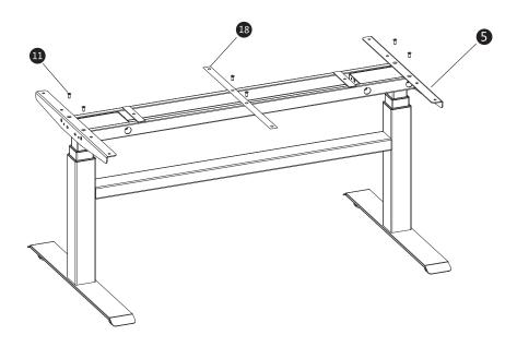
4. Fix the hanger fixture to both sides of the side bracket, fix it firmly with M6X18 screw and fix with M10 inner hexagonal cylindrical head screw to ensure locking.
