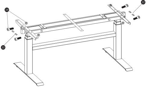
5. Place the trunk hook as one left and one right, merge the trunking from the bottom to the top, and lock it with M4 head cap screws.
