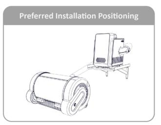
(note: for longer life of the unit, air-conditioning unit should not be placed lower than the ICU unit)
